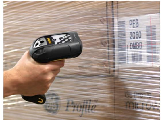
The DS3500 Series delivers blazing performance on virtually any bar code — including 1D and 2D, DPM and IUID serialized bar codes; damaged and poor quality codes; and even codes buried under shrinkwrap. Designed for scanning in noisy manufacturing environments, the DS3500 Series provides three types of feedback to indicate a successful scan — visual, audio and tactile.
